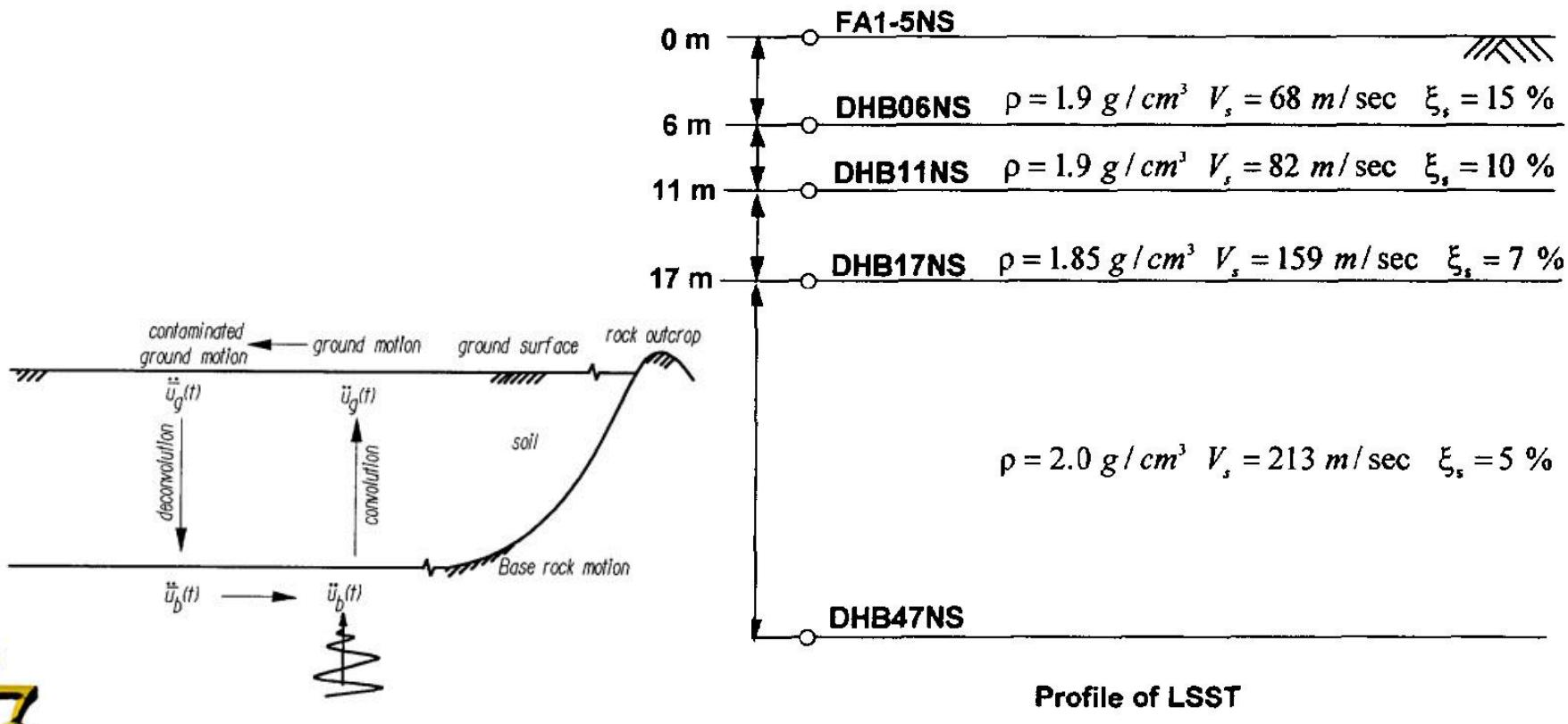
**Fig. 12.** Soil profile of the far-field at the LSST site.
