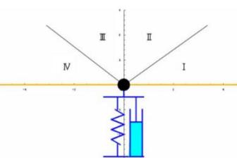
Figure 2. An infinite string with a mass, spring, and damper at the origin.
