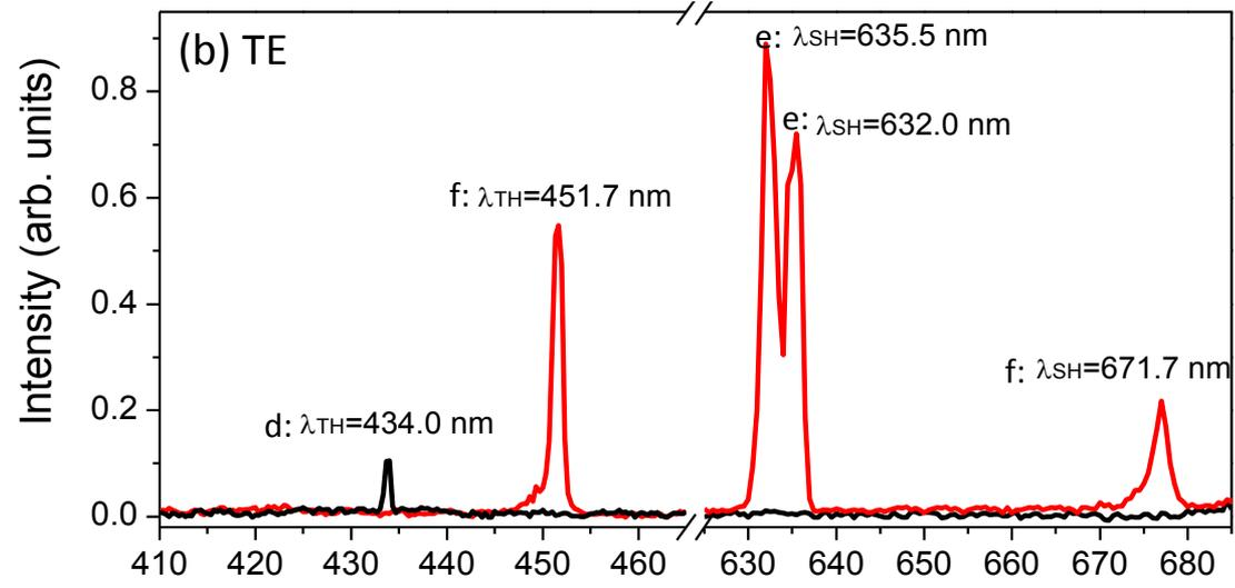
→ Comparing with a sample without WGS, the SHG and THG output can be enhanced by 1000 times !
