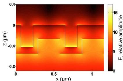
**RWG can produce very sharp guided-mode resonance (GMR) !**
