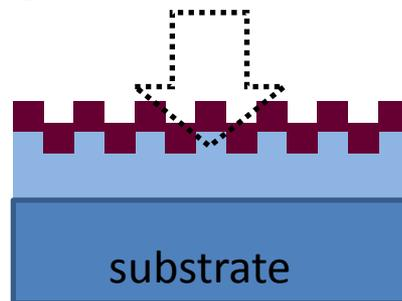
**Photonic crystal substrate (resonant waveguide grating, RWG)**
