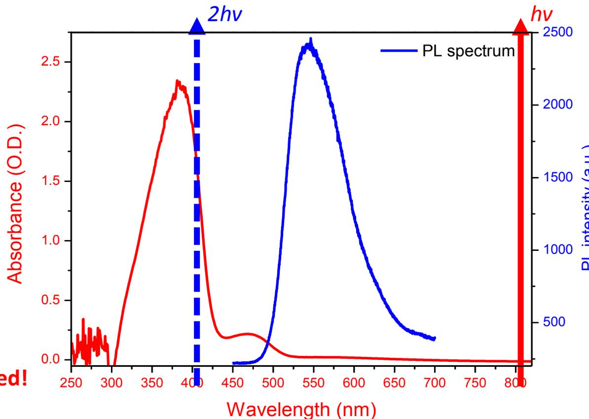
PL spectrum of PFO sample pumped by two photon excitation !
