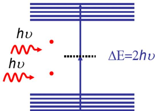
To generate PL signal, higher two-photon excitation intensity is required!
