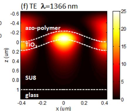
**High SHG and THG output are caused from the strong local field at the interface of an azo-polymer layer and TiO<sub>2</sub> !**
