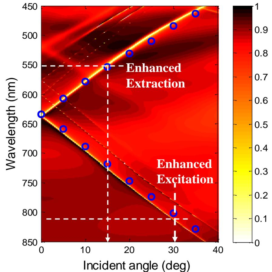
1. GMR at  $\theta=31^\circ \sim 32^\circ$  can be matched with excitation wavelength (810 nm) !
